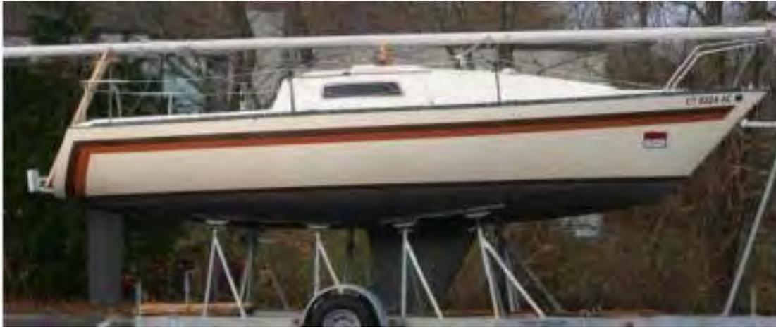
The Sj 7.7 is 'trailerable', but as with any boat with a 4 ft draft and over 9 ft beam, prudence and the proper permits are required. Around 210 San Juan 7.7's were made over its production run, many with the inboard OMC saildrive propulsion. A few were outfitted with single cylinder 7 hp diesel inboards.
